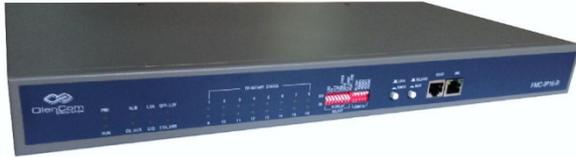
FMC-IP16-R is the IP over TDM converter, which supports the conversion from MAC frames to 1 – 16 E1 lines. The maximum bit rate is 31.68Mbps (16E1 lines). With different LAN card, E1 card and power card, it can meet various requirements. It not only provides alarms and status of the E1 line and Ethernet interface together with advanced management functions, such as, throughput statistic of the Ethernet, but also supports the Unification Network Management via SNMP and CLI commands.
